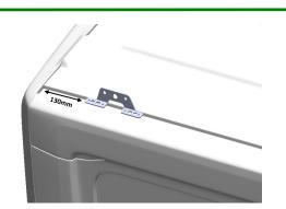
Mark the 5mm rivet holes in each side of the mounting lug & drill with a 5mm drill bit.
