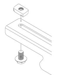
**NOTE-**Ensure attache the channel nuts and bolt to correct mounting slot.
