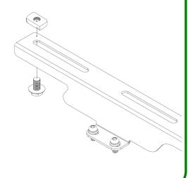
**NOTE-**Ensure attache the channel nuts and bolt to correct mounting slot.
