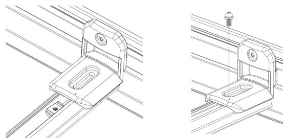
NOTE-Ensure the channel nuts are 90 degrees to the channels.
